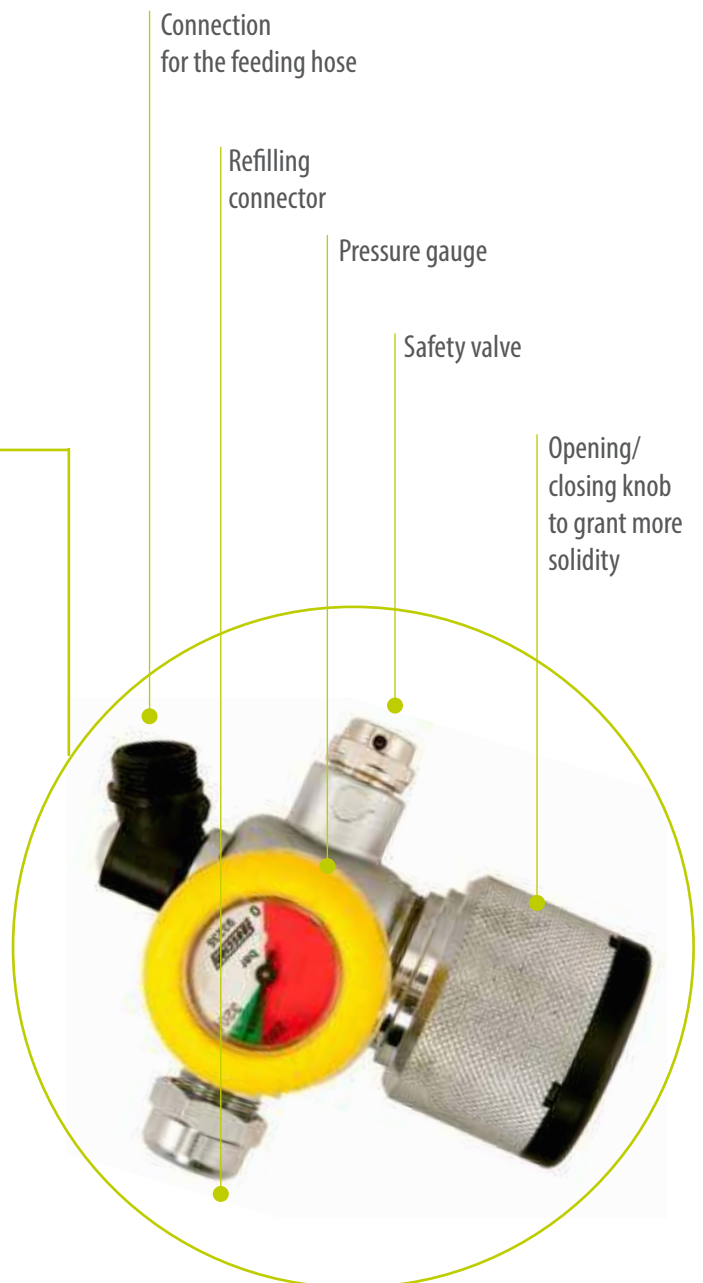
Brass alloy nichel plated pressure reducer
